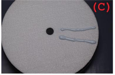
**Tip:** When the pads are new and dry do 5-10 simple light repairs to warm up the pad and build up the Poli-con on the pad. After that the pad will be a lot more effective to remove deeper scratches.
