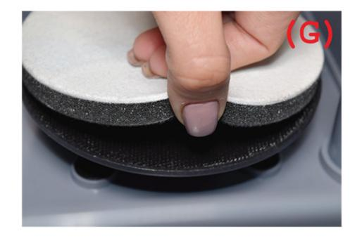
For maximum use of the pad and for best results, we recommend that you wash the pad after 200-250 repairs, or when the surface becomes sticky.
